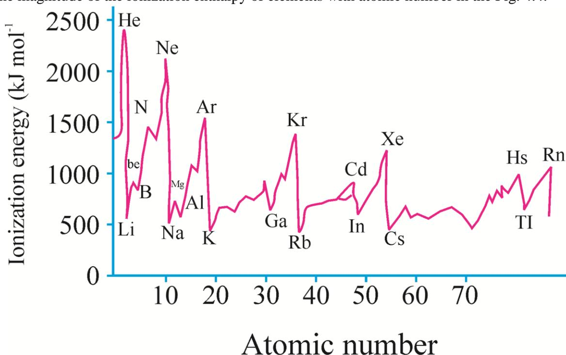
**Fig. 4.4 :** Variation of ionization enthalpy of elements.
