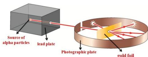
**Fig. 3.2:** Schematic representation of Rutherford's  $\alpha$ -particle scattering experiment.
