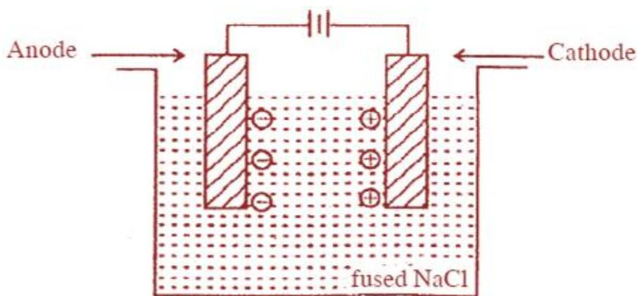
**Fig. 15.3: Electrolytic Cell**
