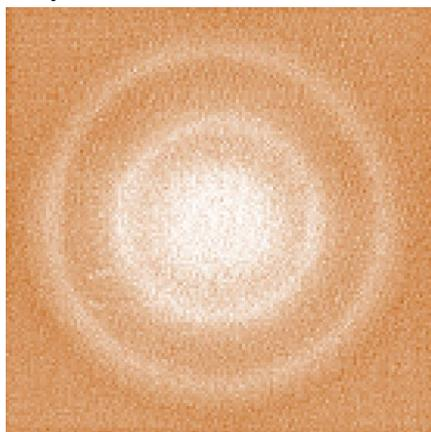
**Fig. 3.13 :** *Electron diffraction pattern from nickel crystal*
