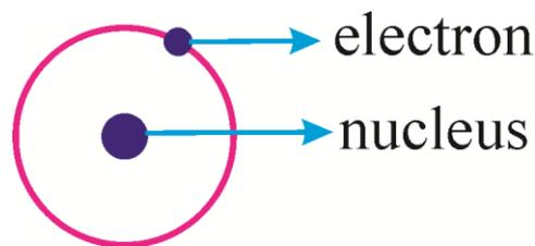
**Fig. 3.3:** Schematic representation of Rutherford's model
