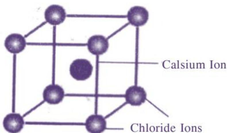
*Fig. 8.17: Caesium chloride structure*
