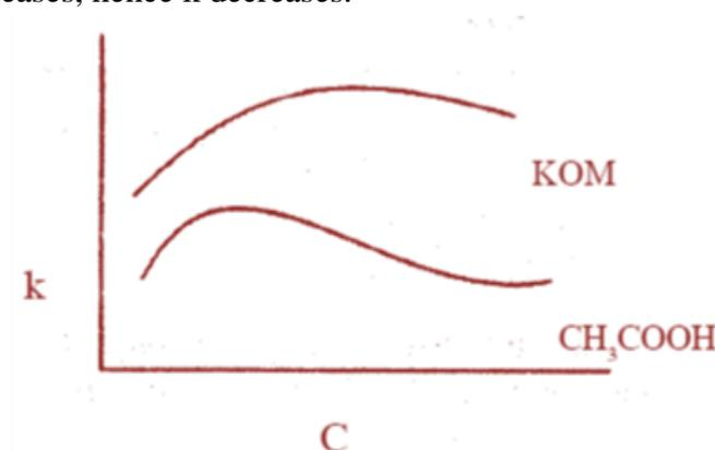
**Fig. 15.1: Variation of conductivity with concentration**
