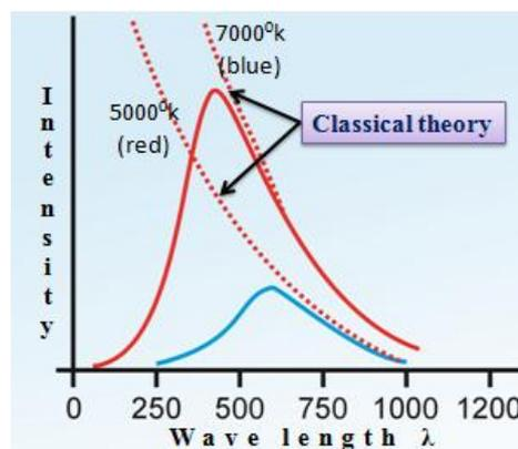
**Fig. 3.9.a Radiations emitted by a black body at different temperatures**
