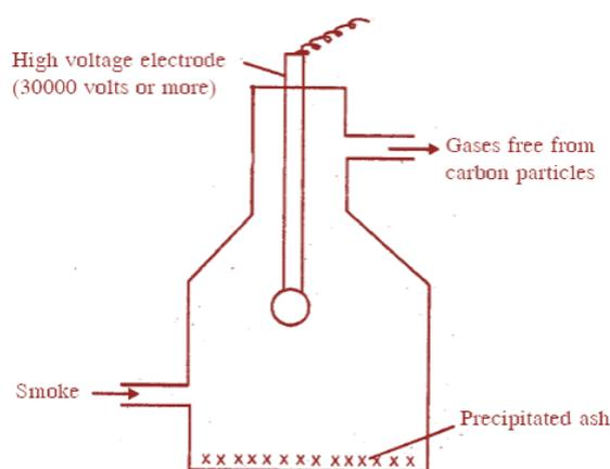
**Fig. 10.8: Cottrell smoke precipitator**
