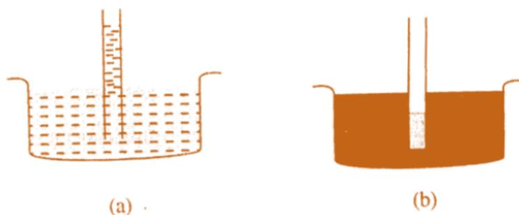
**Fig. 7.7: Capillary Action**
