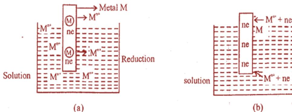
**Fig. 15.7: Metal placed in a solution of its ions**
