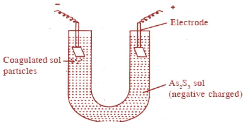
**Fig. 10.7: A set up for Electrophoresis**
