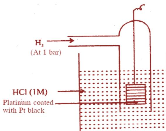
**Fig. 15.8: Standard Hydrogen electrode**
