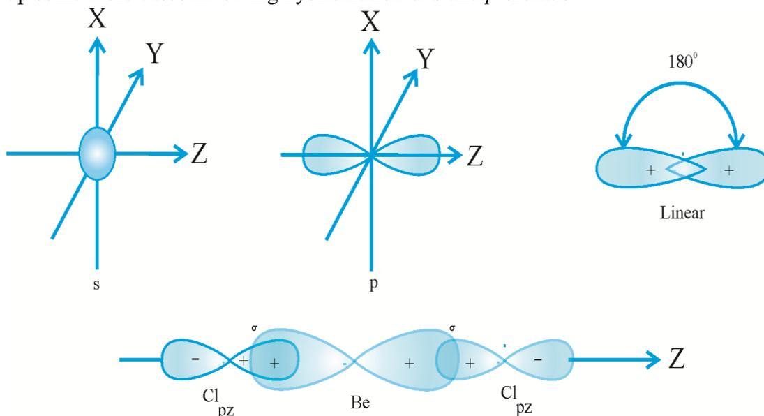
**Fig. 5.2:** Formation of  $\text{BeCl}_2$ ;  $sp$  hybridization
