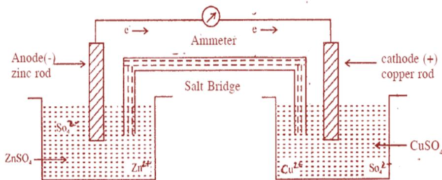
**Fig. 15.6: Daniell cell having zinc and copper electrodes**
