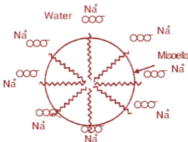
Fig. 10.1: Aggregating of  $RCOO^-$  ions to form a micelle.
