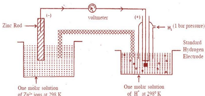
**Fig. 15.9: Measurement of standard electrode potential of Zn/Zn<sup>2+</sup> electrode**
