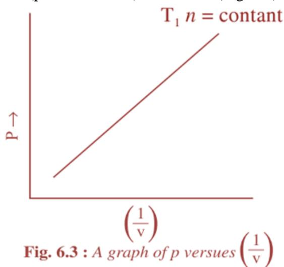
**Fig. 6.3 :** A graph of  $p$  versus  $\left(\frac{1}{v}\right)$
