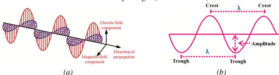
**Fig. 3.6 :** (a) An electromagnetic wave showing electric and magnetic fields travelling in planes perpendicular to each other and also to the direction of propagation
