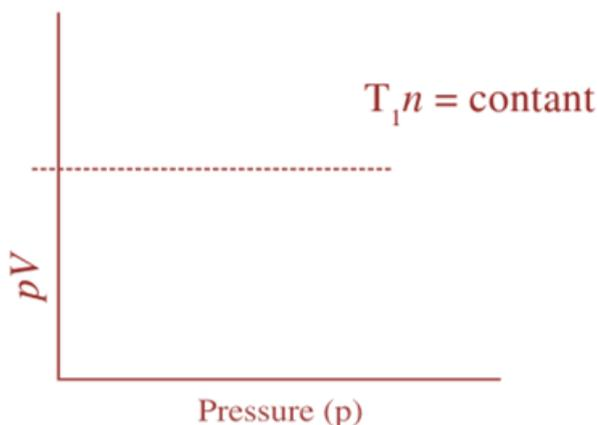
**Fig. 6.4 :** A graph of  $pV$  versus  $p$
