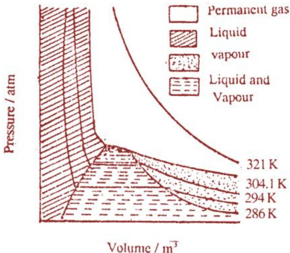
Fig. 6.9: Isotherms of carbon dioxide
