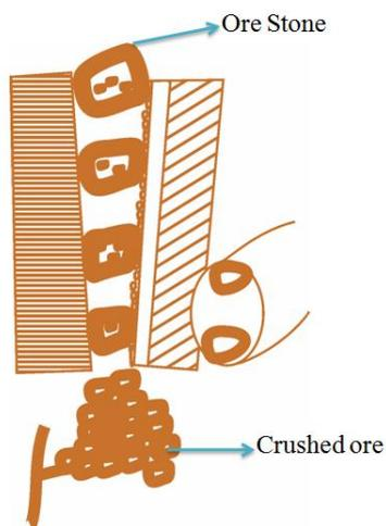
Fig. 18.1 :Jaw Crusher
