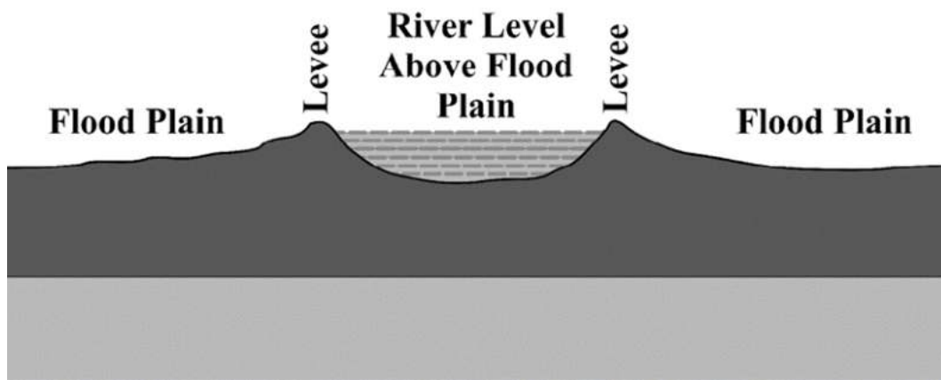
Fig. 4.4 Flood Plain and Levees
